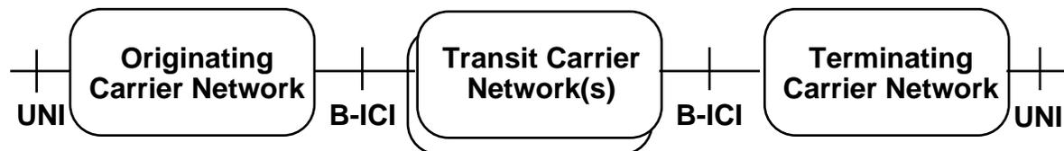
**Figure 12.8 Example Reference Configuration**
