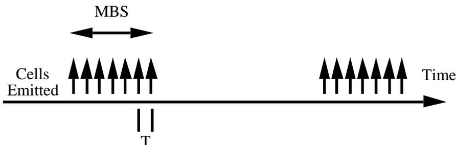
**Figure 5.1 Traffic Source Model Used to Provide Reference Traffic Load Type 3**
