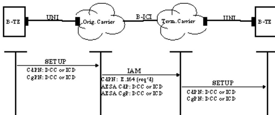
**Figure 1 Coding of IAM across B-ICI: Originating Carrier Generates an E.164 CdPN**
