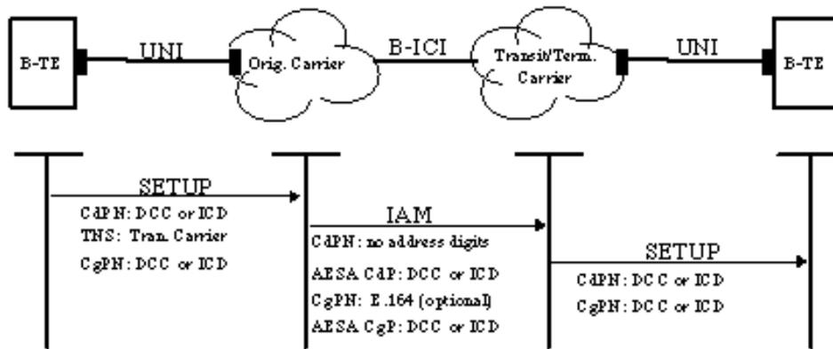
**Figure 3 Coding of IAM across B-ICI: Originating Carrier uses TNS and Generates a CdPN with no Address Digits**
