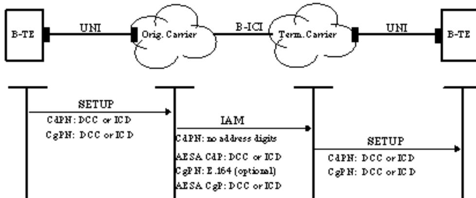
**Figure 2 Coding of IAM across B-ICI: Originating Carrier Generates a CdPN with no Address Digits**
