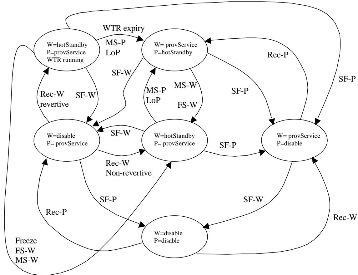
State diagram A-2. The diagram shows the allowed state combinations and examples of transition signals for the working and protection entity.
