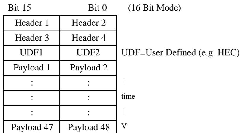
**Figure 8. Cell Format in 16-bit mode**
