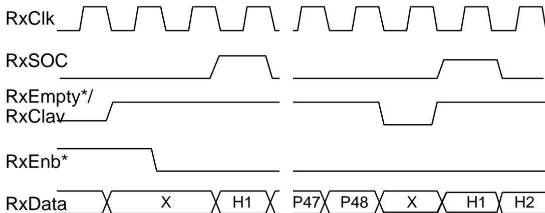
**Figure 7. RxEmpty\*/RxClav Timing**
