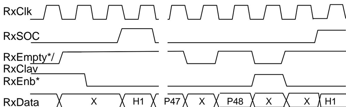
Figure 6. Receive Timing for Octet or Cell-Level Handshake
