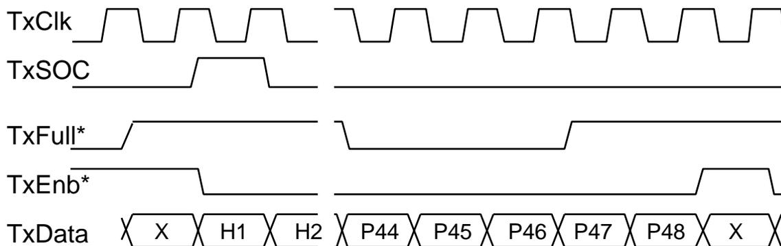
**Figure 3. Transmit Timing for Octet-Level Handshake**
