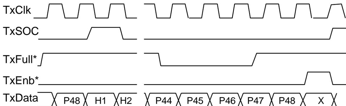
**Figure 4. Transmit Timing for Cell-Level Handshake**
