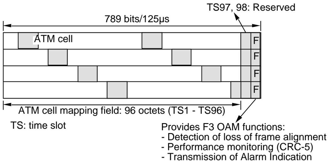
Figure 2-3 Frame structure for 6,312 kbps used to transport ATM cells
