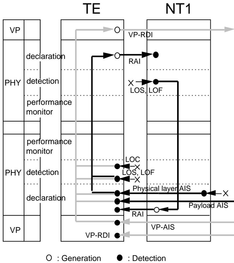
Figure 2-4 Maintenance signal flow
