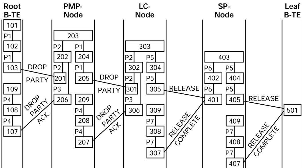
**Figure C-5 Information Flows for a Local Acknowledgement of DROP PARTY from an Existing Point-to-Multipoint Call**
