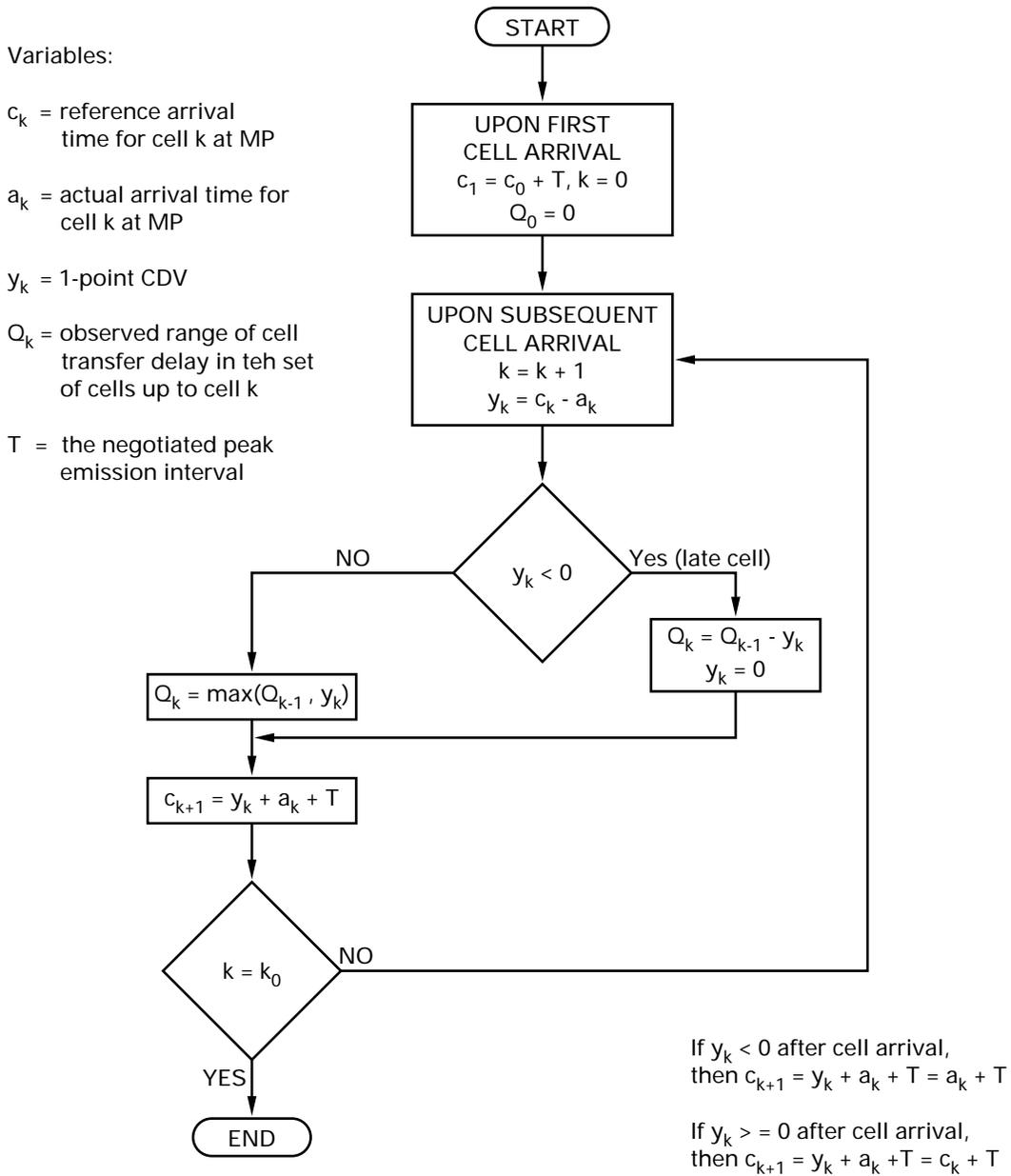
Figure A-2 Estimation of 2-point CDV from 1-point CDV for Connections providing CBR service
