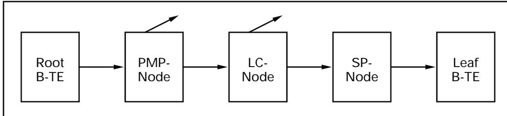
*Figure C-3 Functional Blocks of a Point-to-Multipoint Call*
