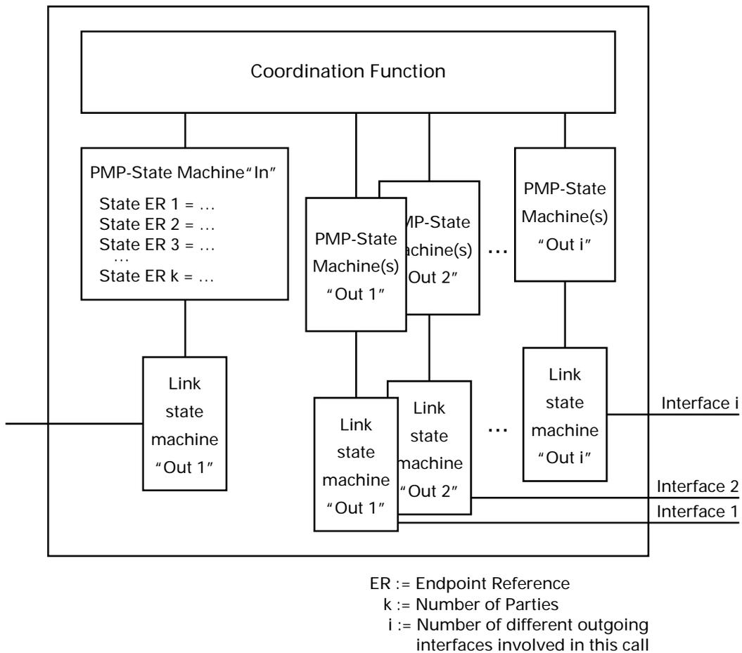
**Figure C-2 State Machines of a Network involved in a Point-to-Multipoint Call**
