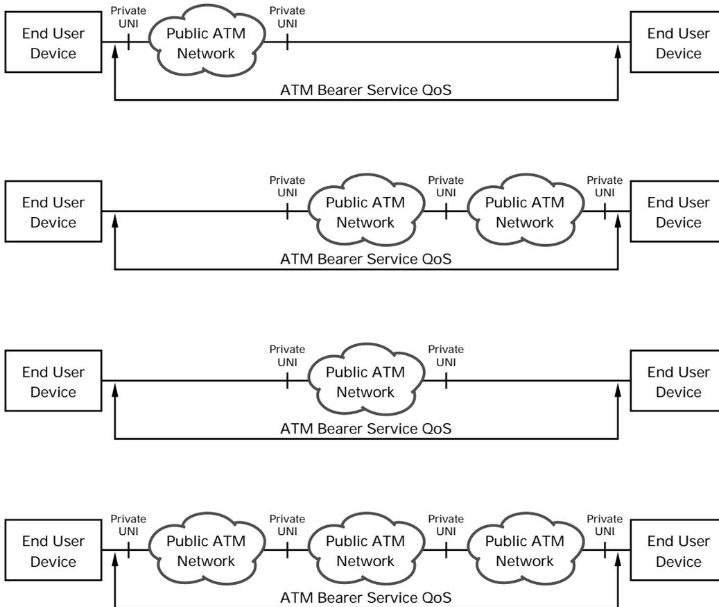
**Figure A-1 ATM QoS Reference Configuration**
