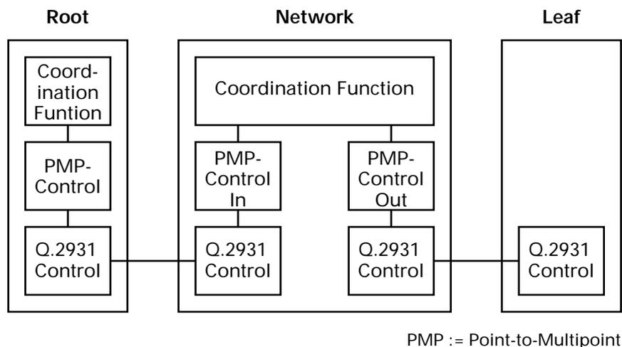
Figure C-1 Control Model with Separated State Machines
