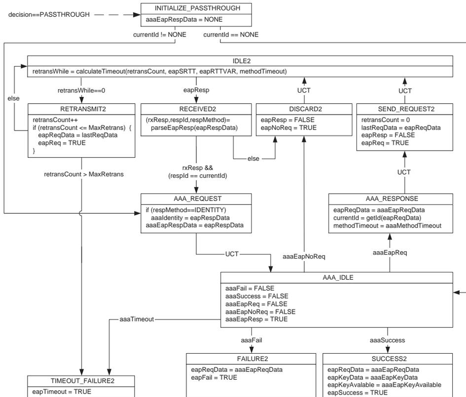
Figure 7: EAP Full Authenticator State Machine (Part 2)
