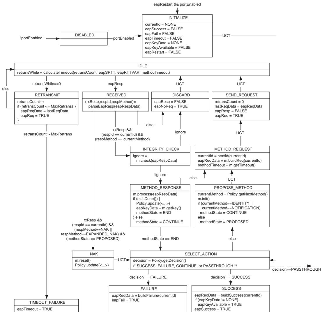
Figure 6: EAP Full Authenticator State Machine (Part 1)
