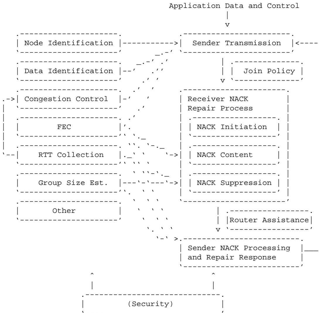
Fig. 1 - NORM Building Block Framework
