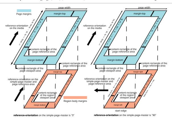
If the block-progression-dimension of the properly stacked region-reference-area is greater than the block-progression-dimension of the region-viewport-area that is its parent, then the constraints on the relationship between the region-viewport-area and the region-reference-area depend on values of the *overflow* trait on the region-master and the kind of flow assigned to the region.
