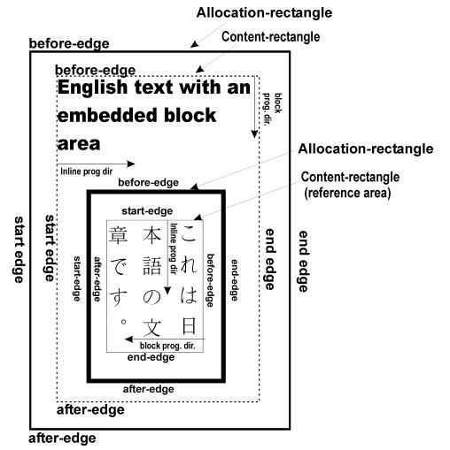
Each inline-area has an *alignment-point* determined by the formatter, on the start-edge of its allocation-rectangle; for a glyph-area, this is a point on the start-edge of the glyph on its alignment baseline (see below). This is script-dependent and does not necessarily correspond to the (0,0) coordinate point used for the data describing the glyph shape.
