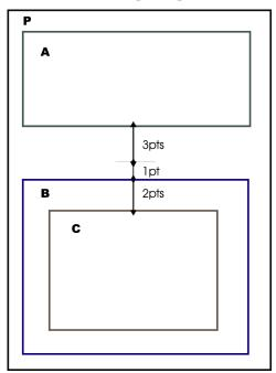
*Example*. In the diagram, if area A has a space-after value of 3 points, B a space-before of 1 point, and C a space-before of 2 points, all with precedence of *force*, and with zero border and padding, then the constraints will place B's allocation-rectangle 4 points below that of A, and C's allocation-rectangle 6 points below that of A. Thus the 4-point gap receives the background color from P, and the 2-point gap before C receives the background color from B.
