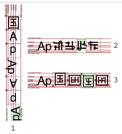
The figure illustrates the positioning of rotated and inverted glyphs in both vertical and horizontal writing-modes. The three examples show first some glyphs typical of the writing mode and then some atypical glyphs in each of the possible orientations, 0, 90, 180 and -90 degrees, in that order. The alignment-point for each glyph is shown as a small "x" whose center is at the alignment-point.
