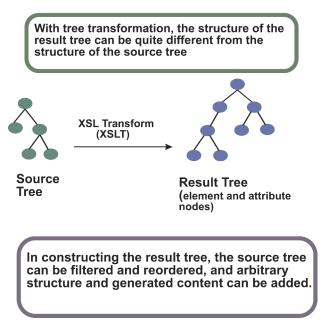
The XSL stylesheet is used in tree transformation. A stylesheet contains a set of tree construction rules. The tree construction rules have two parts: a pattern that is matched against elements in the source tree and a template that constructs a portion of the result tree. This allows a stylesheet to be applicable to a wide class of documents that have similar source tree structures.
