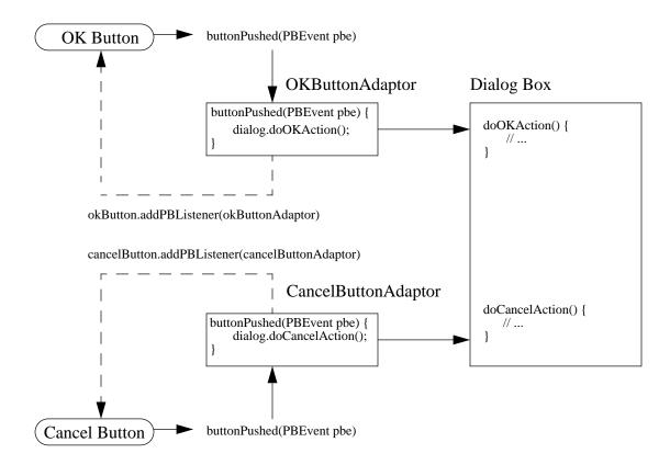
In the example (see the diagram and code below) a DialogBox object has two push buttons "OK" and "Cancel", both of which fire a *buttonPushed(PBEvent)* method. The DialogBox is designed to invoke the methods, *doOKAction()* when the "OK" button fires, and *doCancelAction()* when the "Cancel" button fires.
