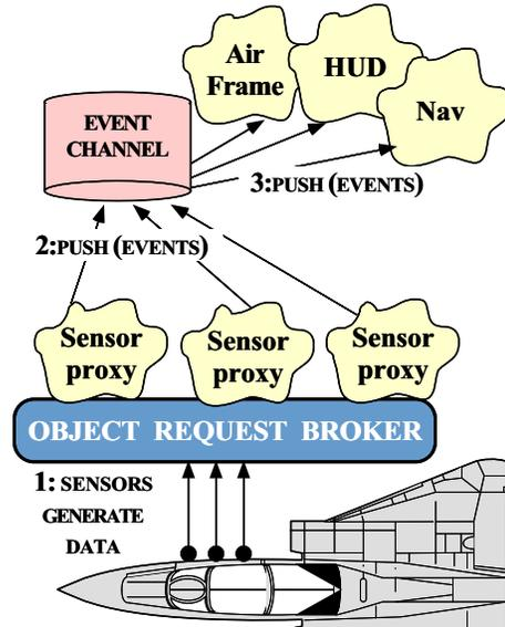
Figure 1: Example Avionics Mission Computing Application
