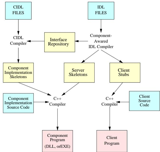
Figure 3: Using IDL and CIDL for component implementation
