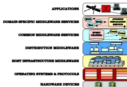
Figure 1: Layers of Distributed Object Computing (DOC) Middleware
