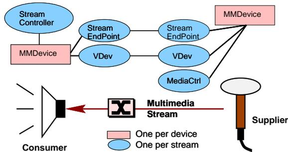
Figure 9: CORBA A/V Streaming Service Components
