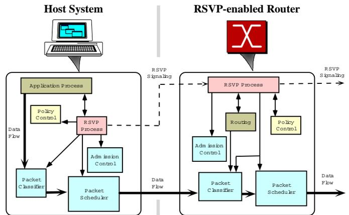
Figure 6: Components in RSVP-enabled Endsystems and Network Elements
