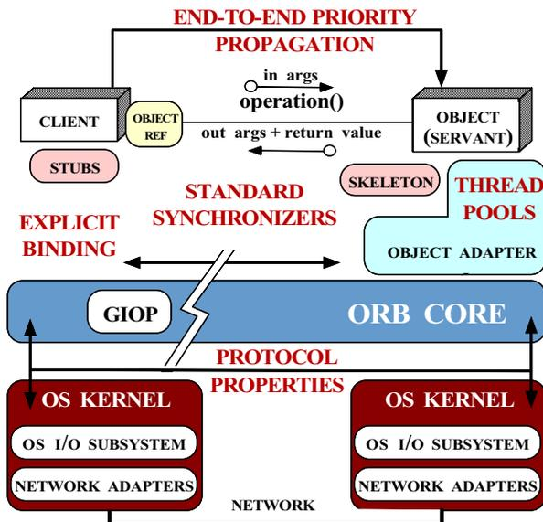
Figure 4: QoS-enabled ORB Endsystem Capabilities in CORBA 3.0
