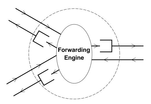
A router contains links, a forwarding engine and queues. Our model included the (deterministic) links and forwarding but not the random, unpredictable, queuing time due to competing traffic.
